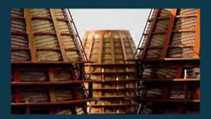
The screen wires are precision-welded to support rods at every junction, guaranteeing a robust and rigid construction. Each basket undergoes a meticulous balancing process before shipping, ensuring prolonged and reliable service.
