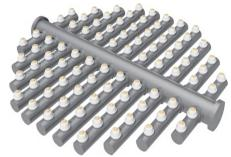
A typical configuration involves placing a header lateral assembly at the top of the vessel to evenly distribute the inlet flow across the bed surface. A second assembly at the bottom of the vessel collects the treated fluid, ensuring even distribution throughout the entire vessel length and cross-sectional area.
