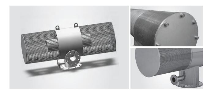
Cylindrical intake screens are fully submerged in the water. They retain larger particles and water life floating in the river and protect pumps and installations further up the production line. The controlled lower slot velocity along the screen surface also reduces the likelihood of impingement and entrainment of marine life.
